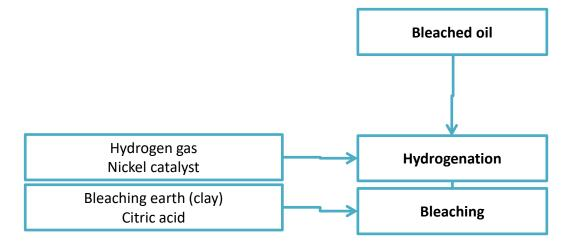
Removes unsaturation by reduing double bonds
