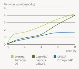
Samples irradiated by low intensity UVA at 35°C with free access to air.
